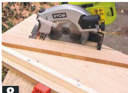
5 Mark veneered MDF sheet and cut pieces to size. Stick masking tape across grain when sawing
